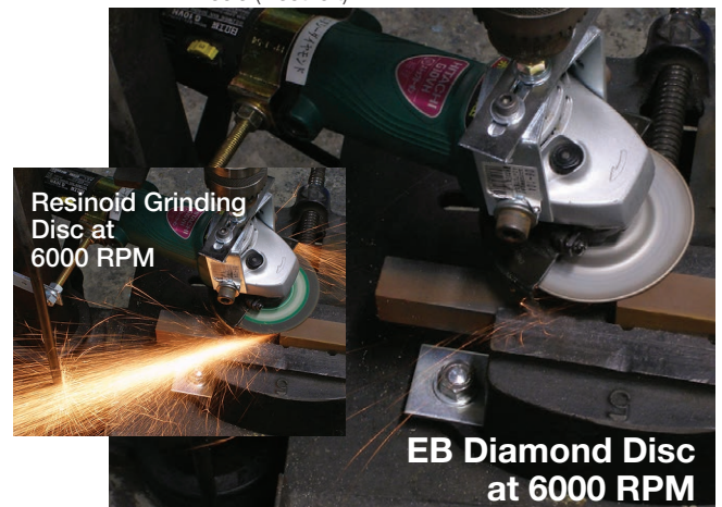
EB diamond grinding discs reduce sparking up to 1/100 of that produced by resinoid grinding wheels (inset left).
