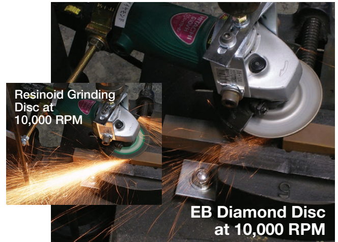
EB diamond grinding discs reduce sparking up to 1/100 of that produced by resinoid grinding wheels (inset left).
